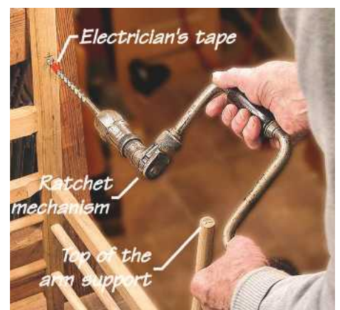
▲ Pic. 9 Aligning the drill for the arm's mortise hole calls for some electrician's tape
